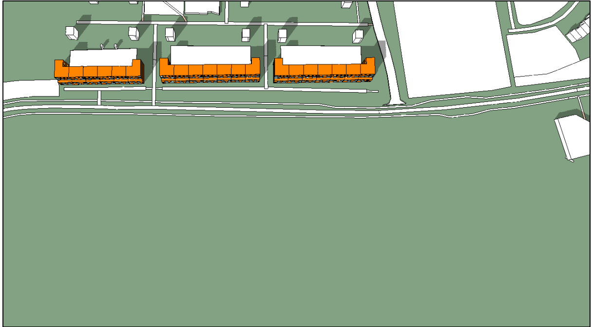
Figure 306. Shadow image on June 21 st at 18:00 of Cedarbrook Apartments without Proposed Development (modelling software)
