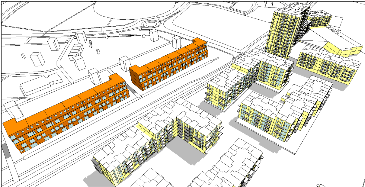
Figure 373. Shadow image on June 21 st at 12:00 of Cedarbrook Apartments with Proposed Development (modelling software)
