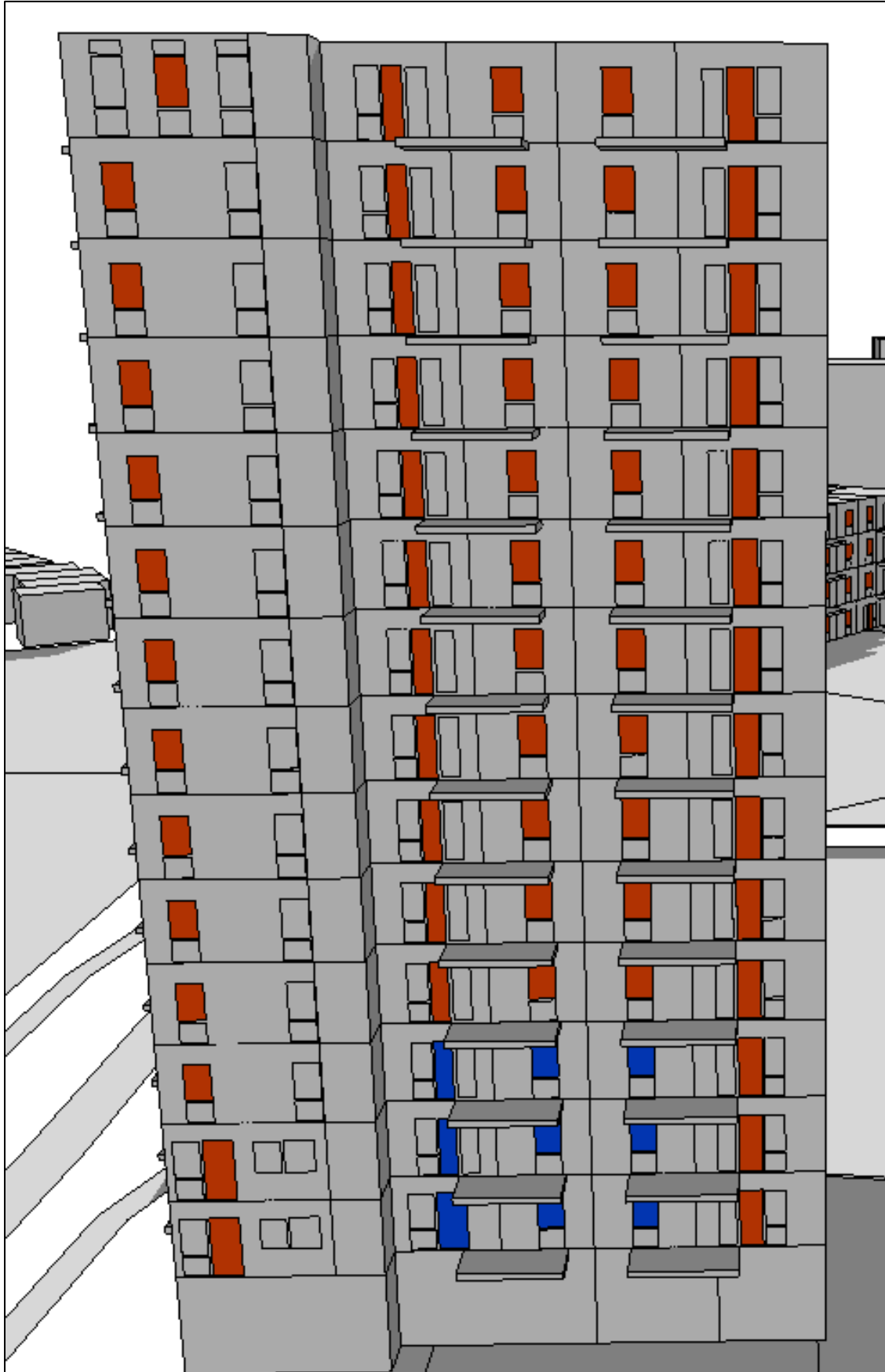
Figure 169. Windows achieving 1.5 hours of sunlight - Northwest elevation of Building 2B (modelling software)
