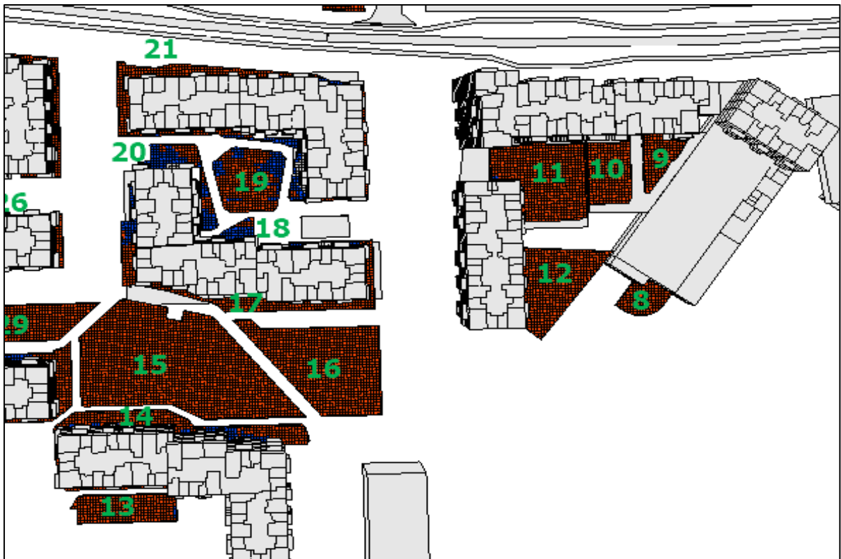
Figure 281. Sunlight on Ground Results for Proposed Amenity Areas near High-Density Buildings (modelling software)
