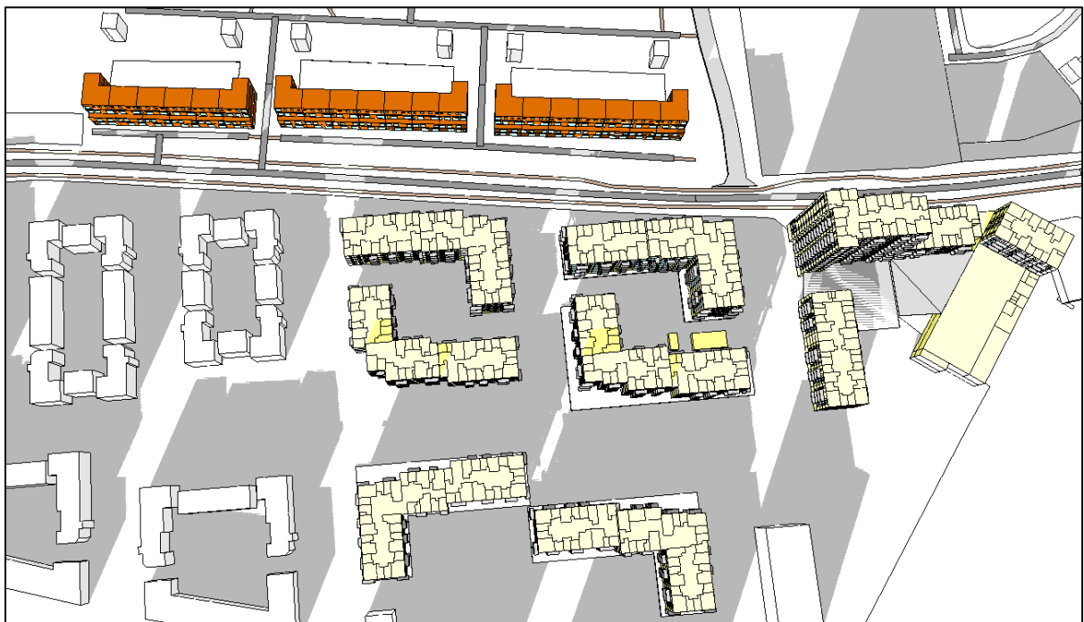
Figure 295. Shadow image on March 21 st at 18:00 of Cedarbrook Apartments with Proposed Development (modelling software)
