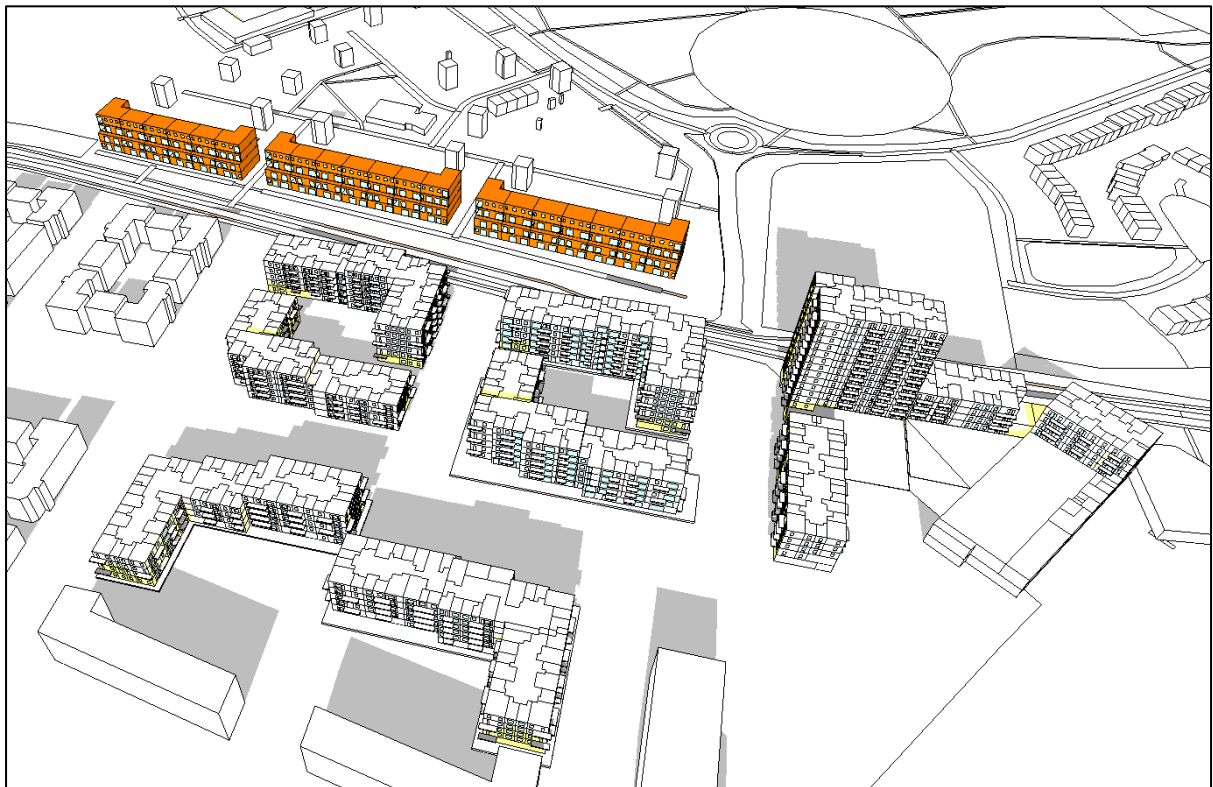
Figure 329. Shadow image on March 21 st at 16:00 of Cedarbrook Apartments with Proposed Development (modelling software)
