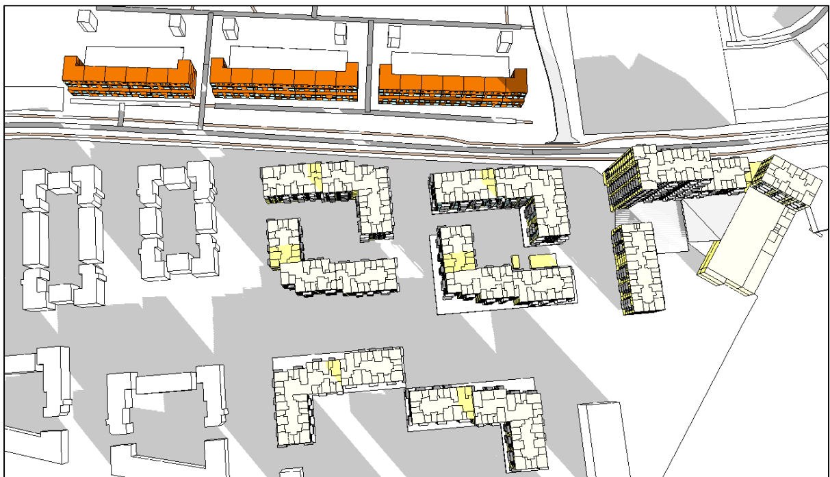
Figure 315. Shadow image on December 21 st at 14:00 of Cedarbrook Apartments with Proposed Development (modelling software)
