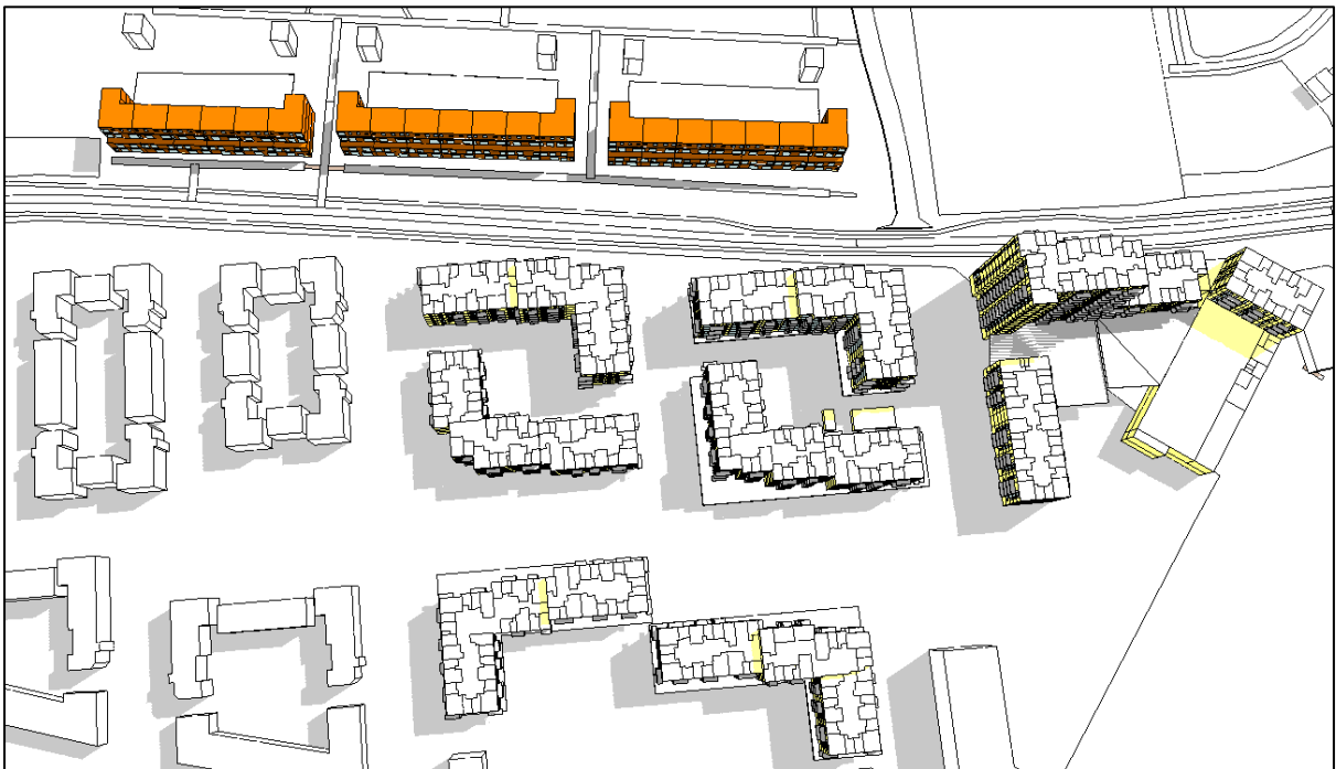
Figure 299. Shadow image on June 21 st at 10:00 of Cedarbrook Apartments with Proposed Development (modelling software)
