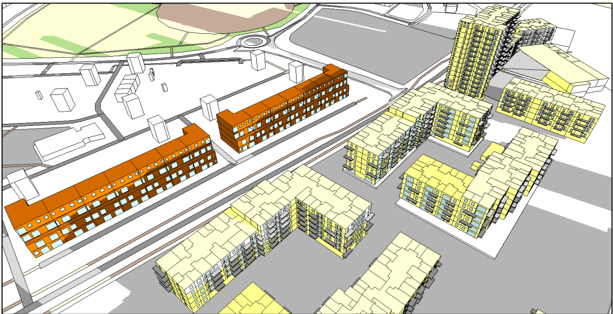
Figure 389. Shadow image on December 21 st at 16:00 of Cedarbrook Apartments with Proposed Development (modelling software)
