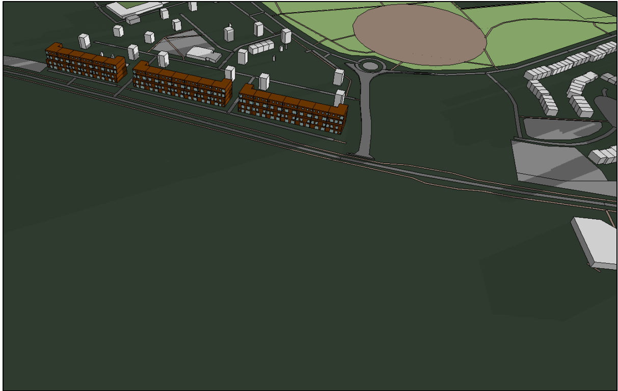
Figure 320. Shadow image on March 21 st at 08:00 of Cedarbrook Apartments without Proposed Development (modelling software)
