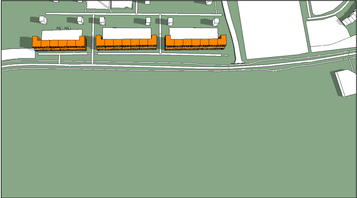
Figure 288. Shadow image on March 21 st at 12:00 of Cedarbrook Apartments without Proposed Development (modelling software)
