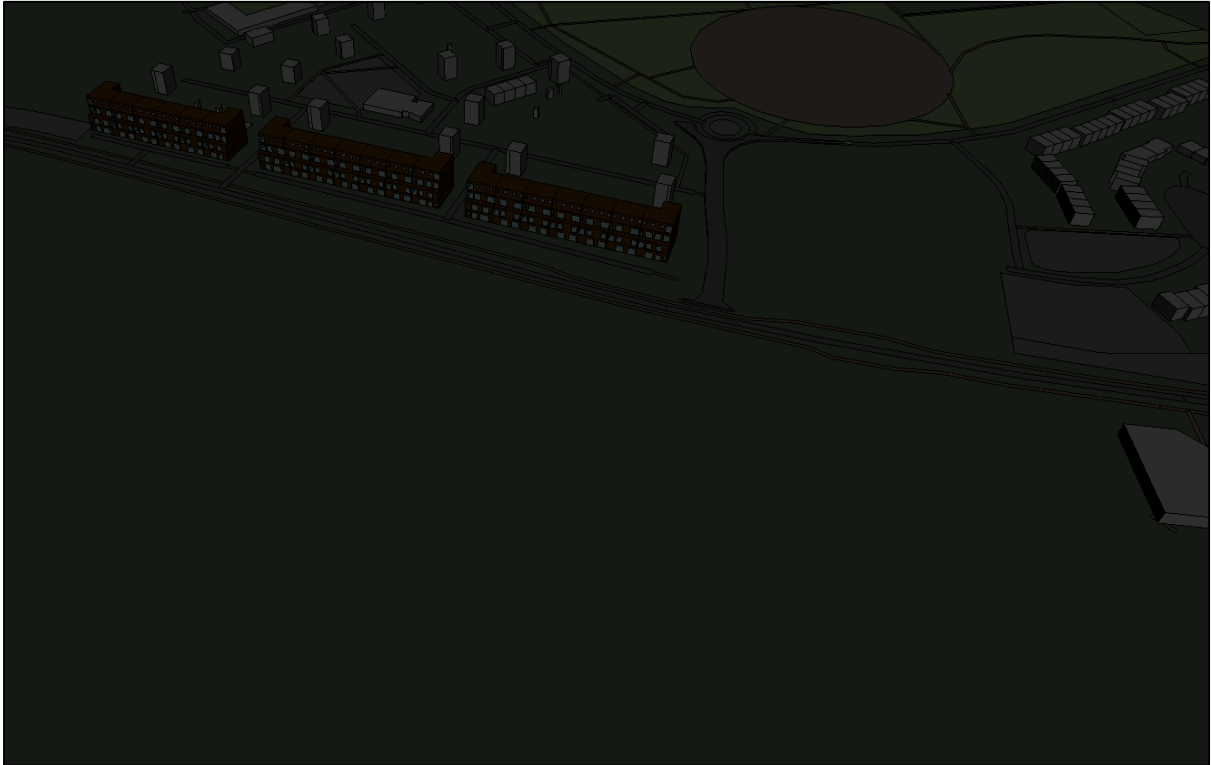
Figure 354. Shadow image on December 21 st at 18:00 of Cedarbrook Apartments without Proposed Development (modelling software)
