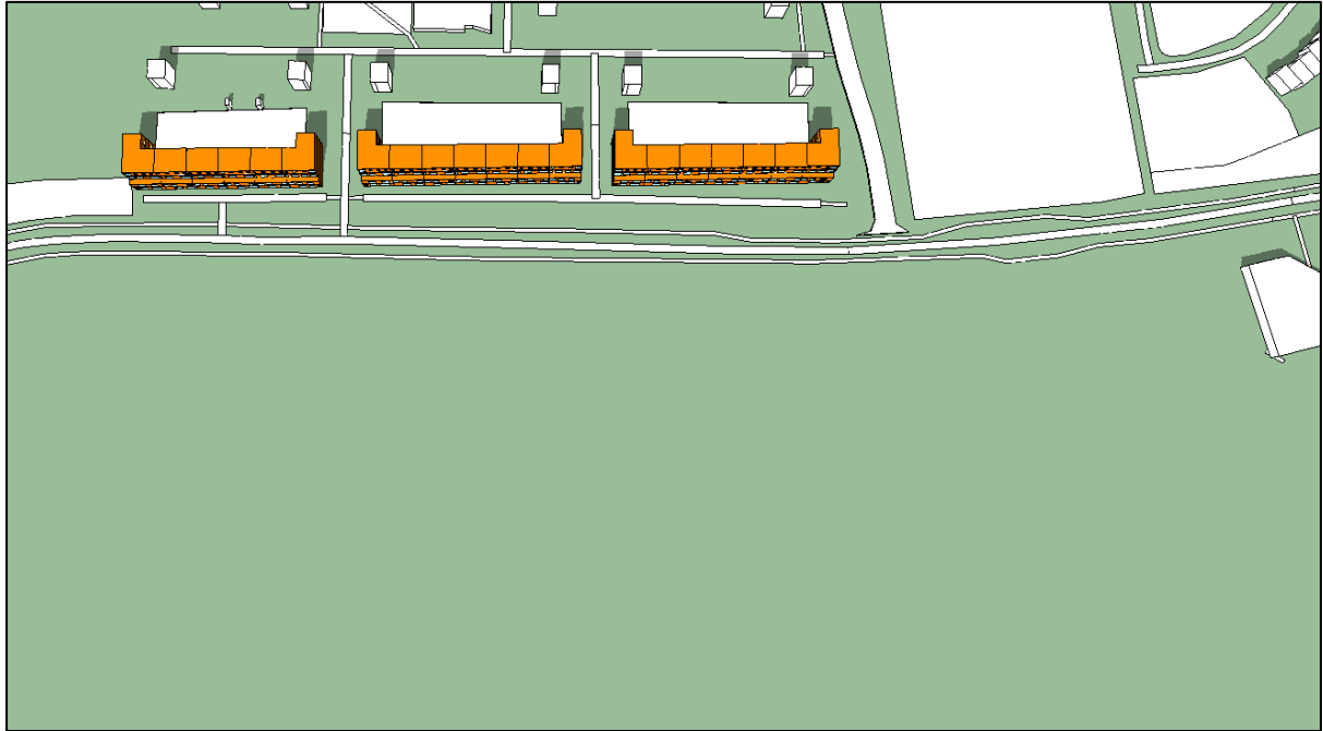
Figure 304. Shadow image on June 21 st at 16:00 of Cedarbrook Apartments without Proposed Development (modelling software)
