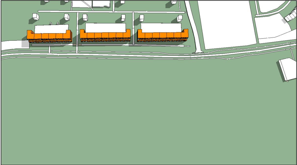
Figure 298. Shadow image on June 21 st at 10:00 of Cedarbrook Apartments without Proposed Development (modelling software)
