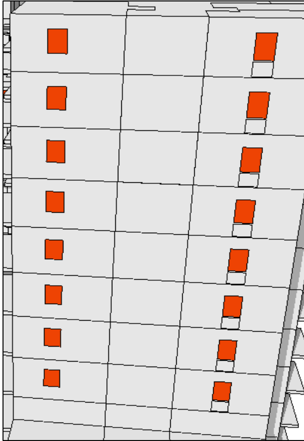
Figure 163. Windows achieving 1.5 hours of sunlight - Southeast elevation of Building 2B (modelling software)
