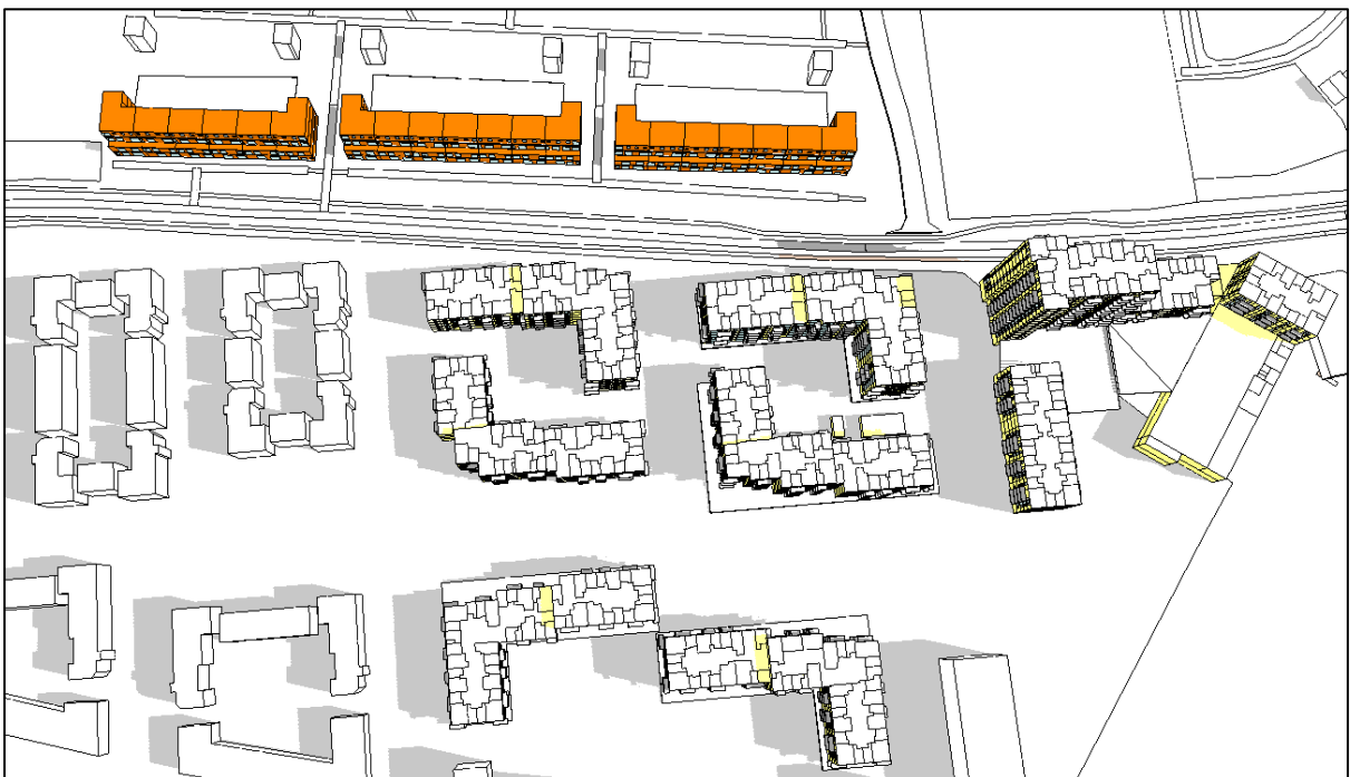
Figure 289. Shadow image on March 21 st at 12:00 of Cedarbrook Apartments with Proposed Development (modelling software)
