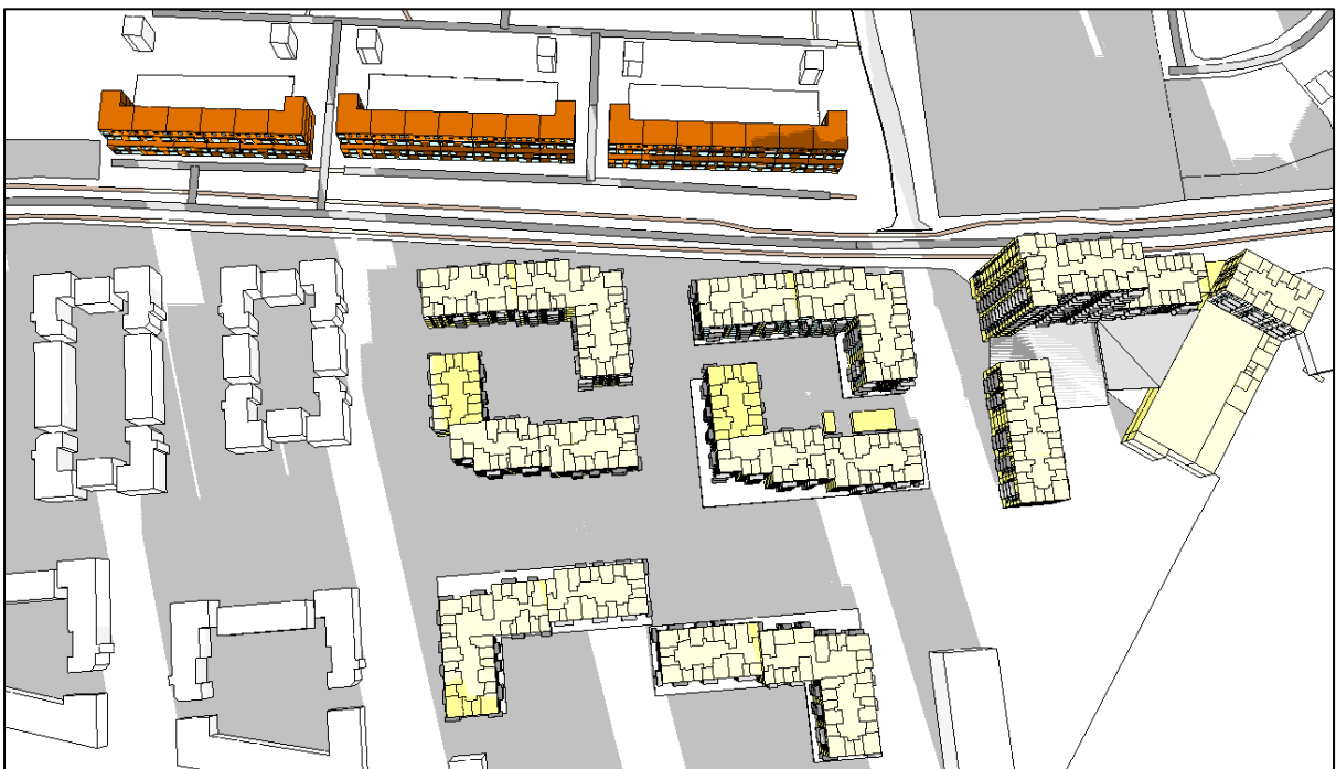
Figure 317. Shadow image on December 21 st at 16:00 of Cedarbrook Apartments with Proposed Development (modelling software)
