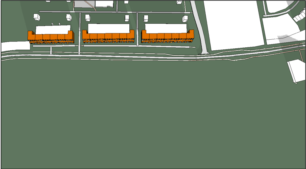
Figure 316. Shadow image on December 21 st at 16:00 of Cedarbrook Apartments without Proposed Development (modelling software)
