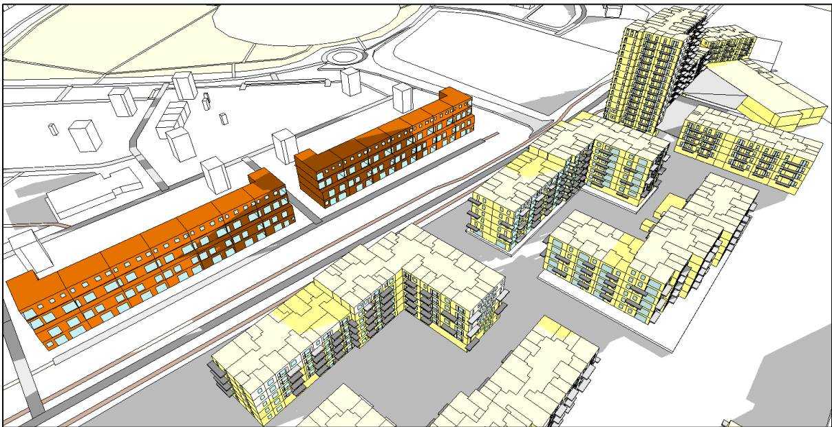
Figure 385. Shadow image on December 21 st at 12:00 of Cedarbrook Apartments with Proposed Development (modelling software)
