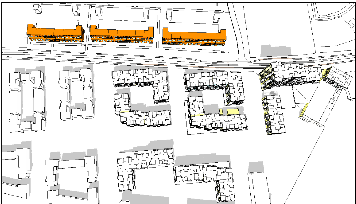
Figure 305. Shadow image on June 21 st at 16:00 of Cedarbrook Apartments with Proposed Development (modelling software)
