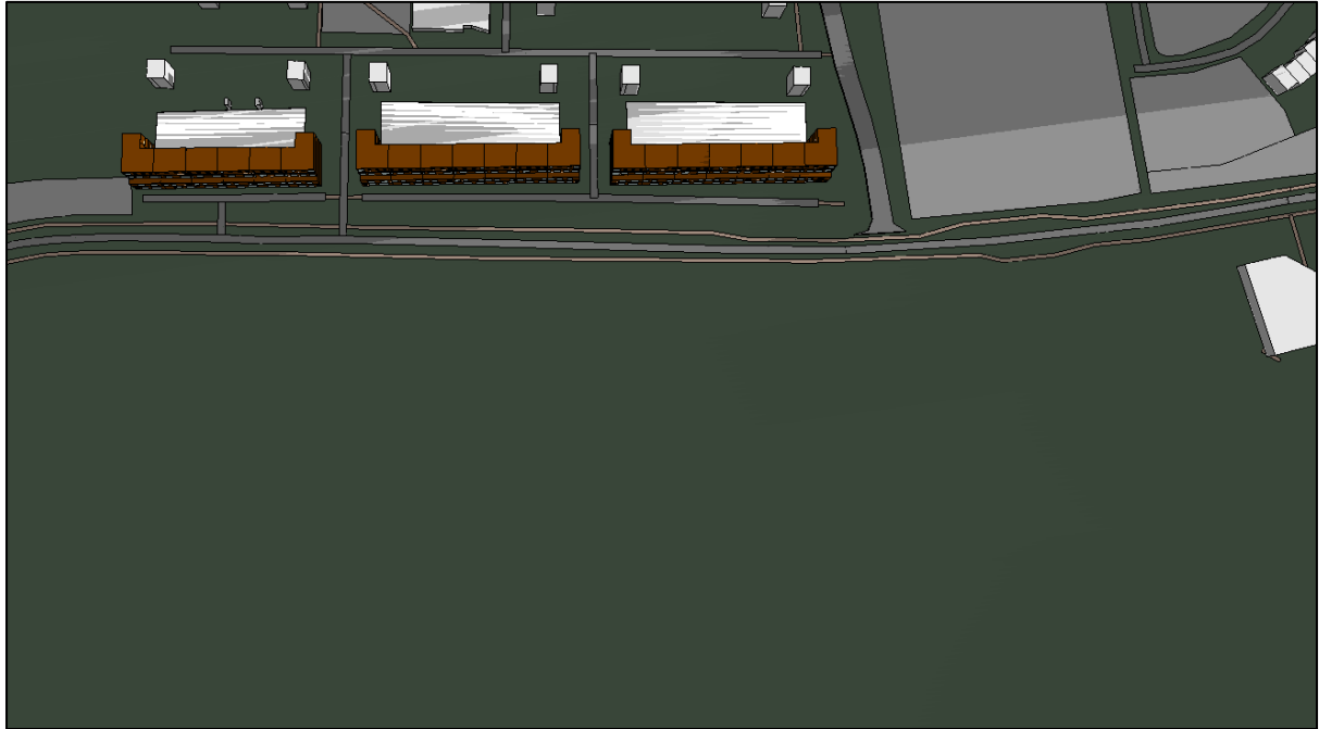
Figure 310. Shadow image on December 21 st at 10:00 of Cedarbrook Apartments without Proposed Development (modelling software)
