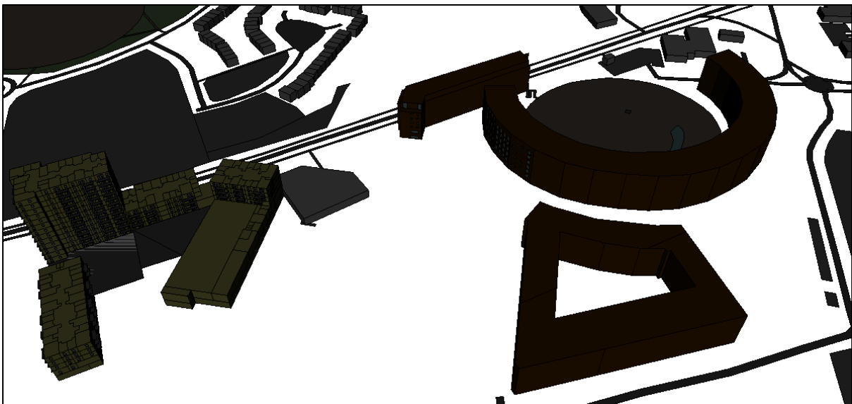
Figure 461. Shadow image on December 21 st at 18:00 of Park West with Proposed Development (modelling software)
