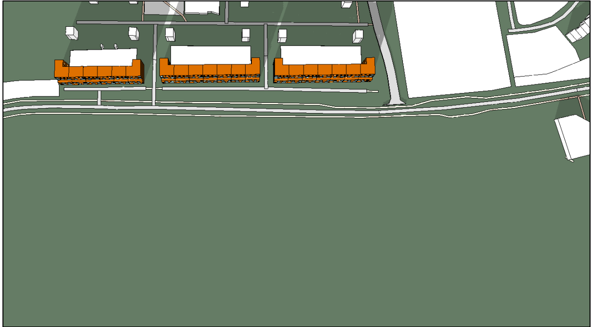
Figure 294. Shadow image on March 21 st at 18:00 of Cedarbrook Apartments without Proposed Development (modelling software)
