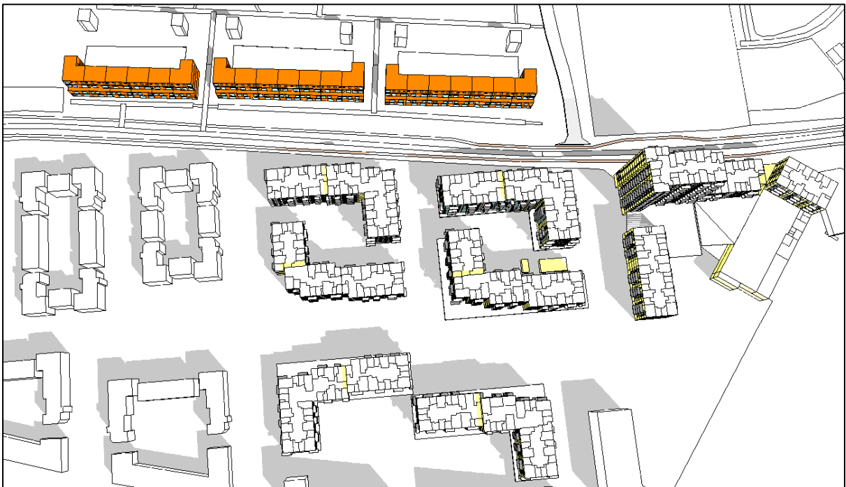
Figure 291. Shadow image on March 21 st at 14:00 of Cedarbrook Apartments with Proposed Development (modelling software)
