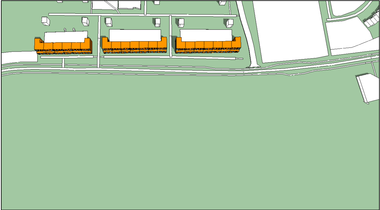
Figure 302. Shadow image on June 21 st at 14:00 of Cedarbrook Apartments without Proposed Development (modelling software)
