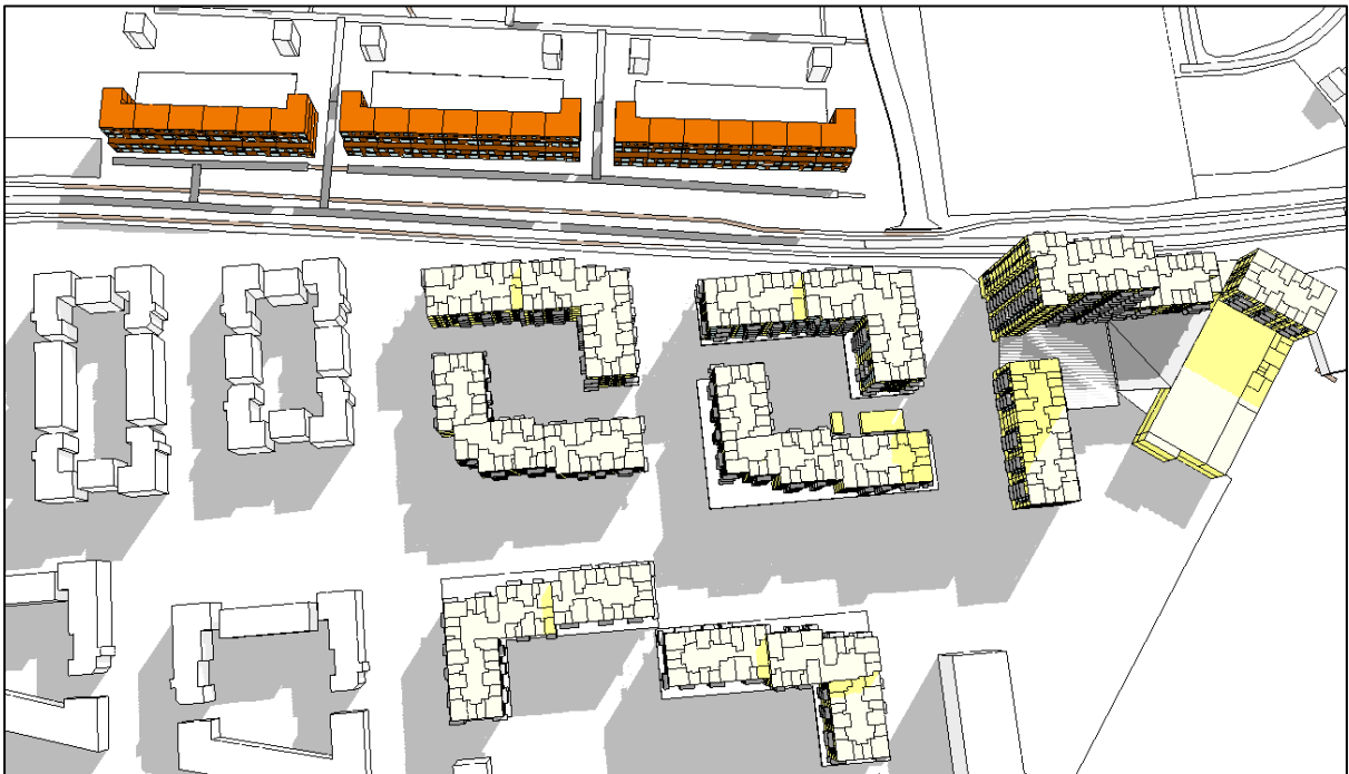
Figure 297. Shadow image on June 21 st at 08:00 of Cedarbrook Apartments with Proposed Development (modelling software)
