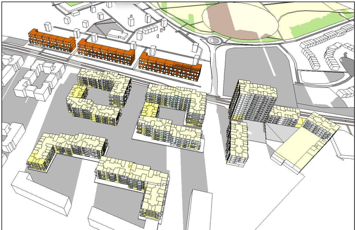
Figure 353. Shadow image on December 21 st at 16:00 of Cedarbrook Apartments with Proposed Development (modelling software)
